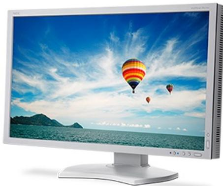
The DCI color gamut lies between Rec.709/sRGB and Adobe RGB and the NEC display has no trouble rendering it. The NEC monitor's fine dot pitch with a satin antiglare coating produces a sharp image, while the backlight consists of green and blue LEDs with the red being created by filters. This extends the gamut beyond what white LED can produce. The MultiSync PA272W sports 14-bit 3D internal programmable
