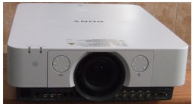
The rest of Sony's feature set includes a standard 1.6:1 zoom lens, the picture by picture (side by side), DICOM support – for displaying medical films and images, and advanced networking with Crestron and AMX support. Geometric related features include lens shift, 360 degree operation, edge blending, and warping and corner
